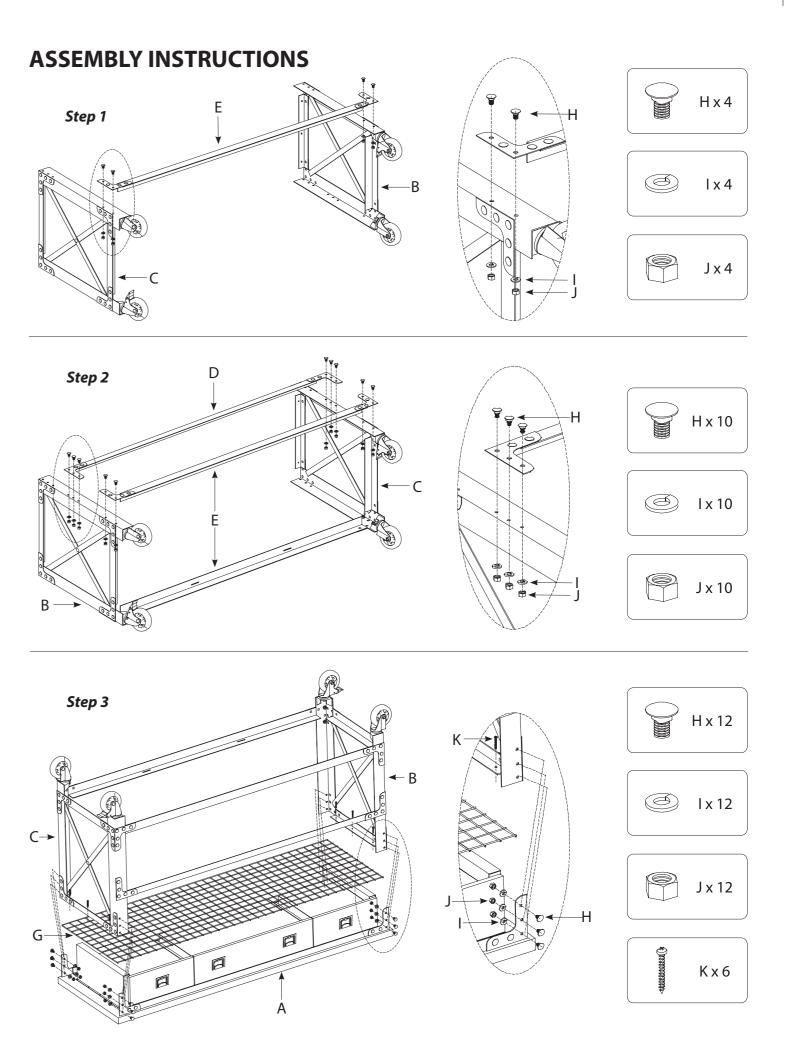
**Note:** Assemble upside down according to instructions. Ensure workbench top is flat on the floor.
